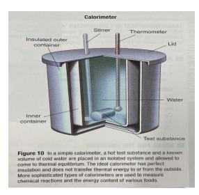
• Carefully insulated so that thermal energy transfer to the external world is kept to a minimum
